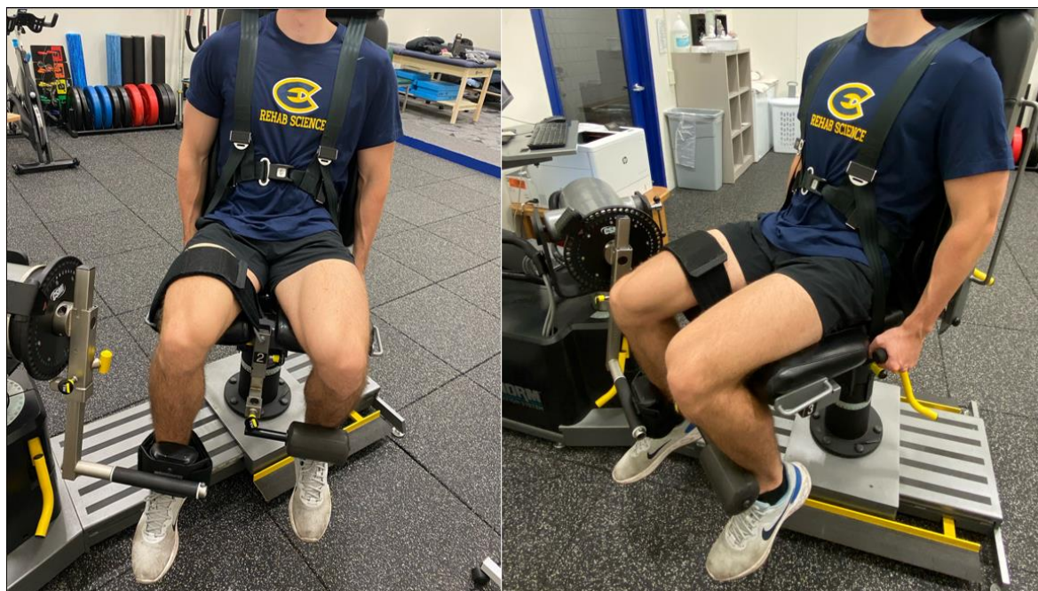
Figure 1. Humac Norm isokinetic dynamometry setup
