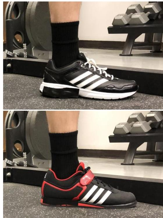
**Figure 1.** The two shoes used in this experiment: the Adidas Falcon Trainer 3 (top) and the Adidas powerlift.2 (bottom). The front edge of each tape strip along the lateral outsole aligns with the foot arch peak.
