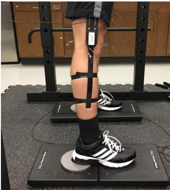
**Figure 2.** Depiction of the cross-training shoe + plate condition with subject standing on the force plates. During the trials where the 2.5 lb. weight plate was used, the weight plate was duct-taped to the rearfoot force plate to ensure the plate was unable to move during the trials (not shown in this picture). This picture also shows how the electrogoniometer was attached to the right leg.
